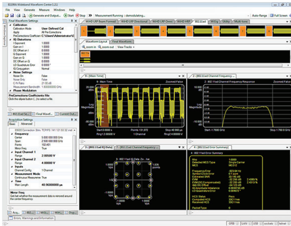
Figure 6. Demodulation of a 802.11ad signal in the 60 GHz band using the Keysight upconverter and downconverter.
