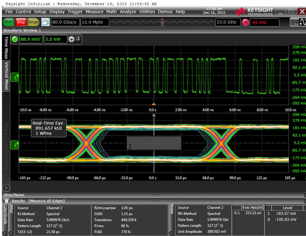
Figure 5. The BER contour is computed statistically from jitter and noise components.
