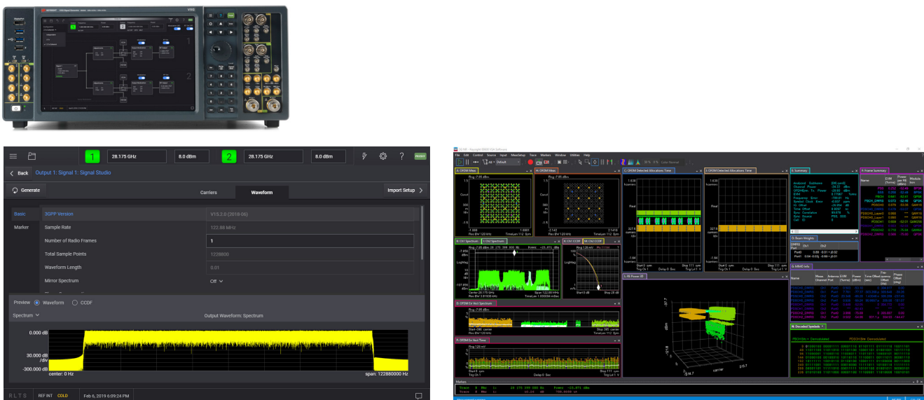
Figure 3. The M9384B VXG Microwave Vector Signal Generator and N7630C Signal Studio software are used for creating a variety of 3GPP 5G NR signals.
