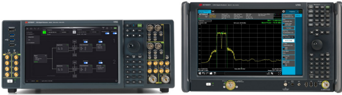
Figure 2. This 5G Testbed configuration supports 3GPP NR signal creation up to 44 GHz with traditional bench top spectrum analysis up to 50 GHz. Both instruments support integrated 1 GHz bandwidth capability.
