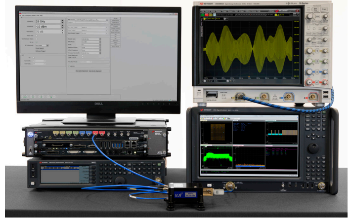
Figure 4. This 5G testbed configuration enables signal generation and analysis of signals between 50 GHz and 110 GHz with very wide bandwidths in excess of +5 GHz. The M8195A arbitrary waveform generator provides direct IF signals to the external mixer, while the N5183B MXG microwave analog signal generator provides the LO for up conversion to mmW frequencies. The N9041B UXA signal analyzer can directly digitize signal bandwidths up to 1 GHz for analysis. The UXA wideband IF output enables +5 GHz bandwidth signal to be analyzed with an oscilloscope.
